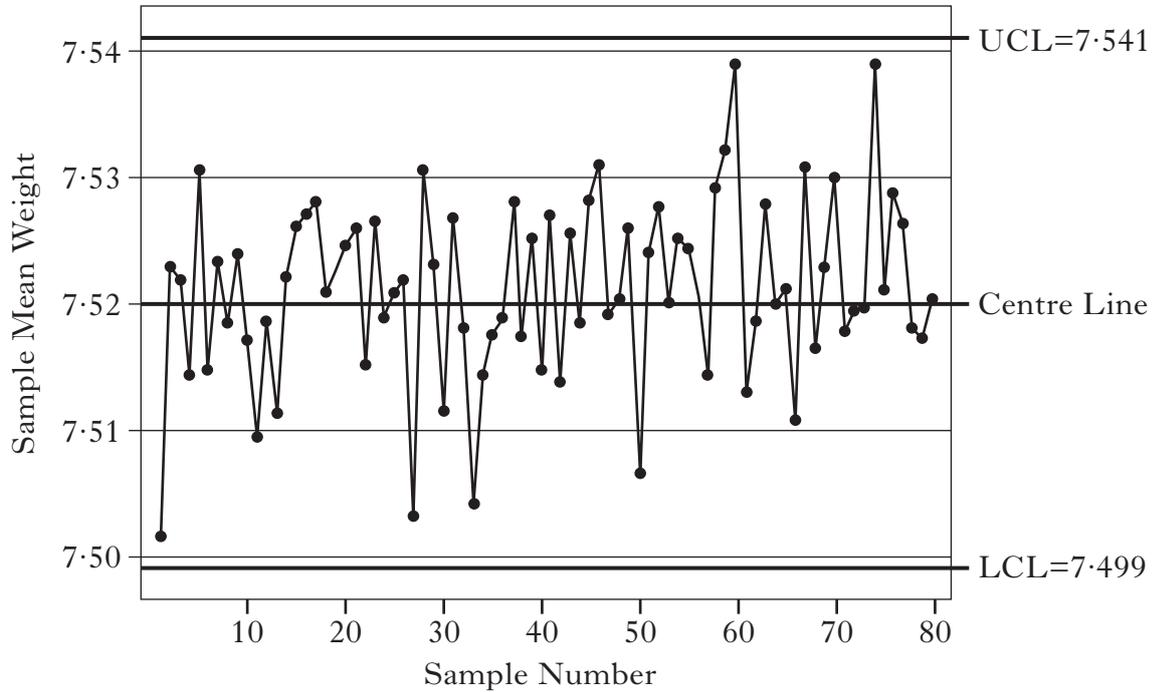
(a) State the features of the plot that indicate that the manufacturing process is behaving in a stable, predictable manner. 1
