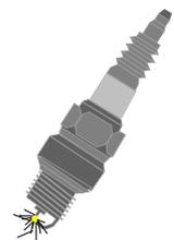
A plug which falls below a *BER* of 80 units should immediately be replaced.
