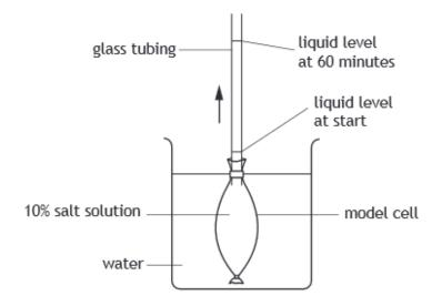
The liquid level in the glass tubing was measured every 10 minutes for 60 minutes.
