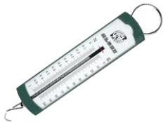
Forces are measured using a Newton balance.
