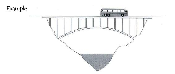
If all the visual components acting on the structure or body were removed and replaced with their force value, a simplified diagram would allow a better understanding of how the forces are affecting the structure.
