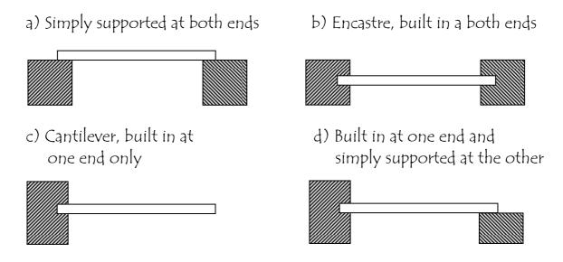
At the point of support, the downward forces acting on the beam are resisted by the forces acting upwards. These upward forces are known as beam reactions, or simply the 'reactions'.
