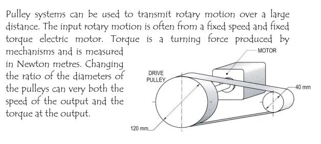
This motor is connected to a pulley of 120mm  $\phi$ . This is the driver pulley. The driven pulley is 40 mm  $\phi$ . To work out the multiplier ratio for a pulley system, use this equation:
