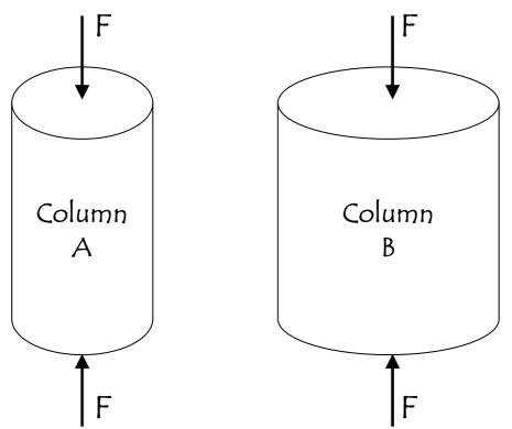
The stress can vary by the force put on it, but also by the size of the structure. For example if the same load is applied to column A and column B, then Column A will suffer more from stress. The reason why is because Column A has a far smaller cross sectional area.
