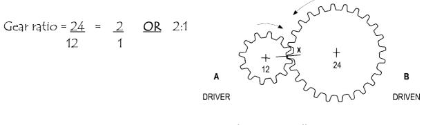
The Driven will be going at <u>HALF</u> the speed of the driver
