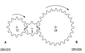
The multiplier ratio for the simple gear train in this diagram is still 2:1. If Gear A still rotates at 100rpm clockwise then the output of Gear B will rotate at 50 rpm clockwise.
