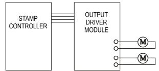
The 'high' and 'low' commands can be used to switch the output pins and control the motors *forward*, *backward* and *halt*.
