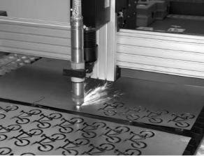
The laser is positioned by motors A and B which are operated by a microcontroller.
