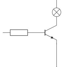
A common way to drive these devices is with a transistor, as shown in the diagram above. In this case the lamp is controlled by the transistor switching on and off.
