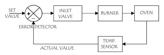
The control diagram includes an *error detector*. It compares the actual value to the set value. If it differs, it changes the input to compensate.
