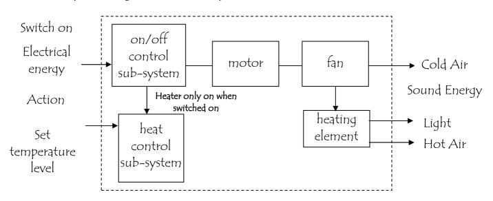
Here the input signal from the on/off and temperature switch is processed to produce the output. The output air is not monitored or adjusted in any way and it is just blown out at whatever temperature the heater warms it to.
