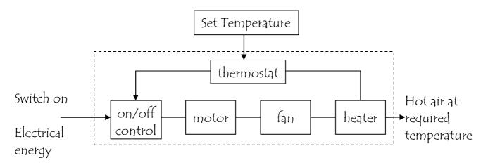
All closed-loop control systems include a sensing sub-system that feedbacks information to the control sub-system. The control subsystem will process this feedback signal and make a 'decision' on whether to alter the output
