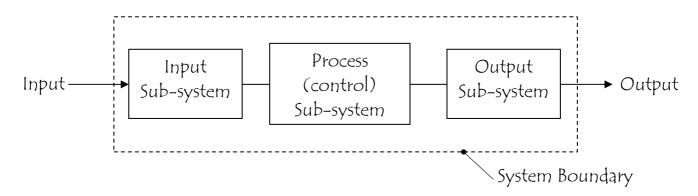
The sub-system diagram shows the *internal* detail of the system. Each box, called a **sub-system**, can be thought of as a system within a system and has its own input and output. The dashed line around the sub-system is called a **system boundary** and this marks the area of interest to us. The 'real world' input and output are shown as arrows entering and leaving the sub-system diagram.
