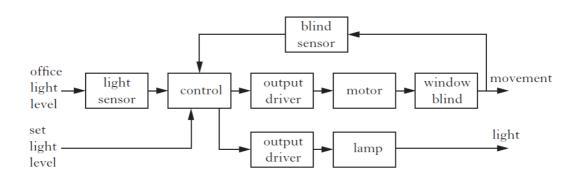
(*a*) (i) Complete the sub-system diagram shown by adding the system boundary.
