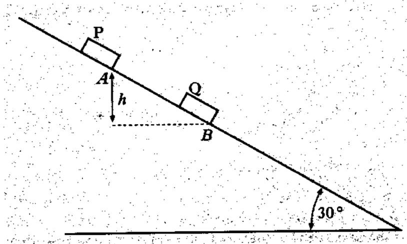
When block  $P$  is released, it slides down, colliding and coupling with block  $Q$ . The combined blocks then move down the rough section of the ramp, coming to rest at a vertical height  $\frac{1}{2}h$  metres below  $B$  ;
