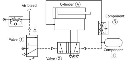
a) Describe, using appropriate terminology, the operation of the pneumatic circuit, shown above.
