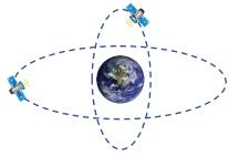
The soy satellite is in polar orbit, 750km directly above the surface of the Earth. IT passes continuously over the Earth's north and south poles as the Earth spins beneath it.
