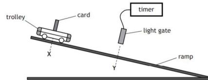
The trolley is released from X and moves down the ramp.
