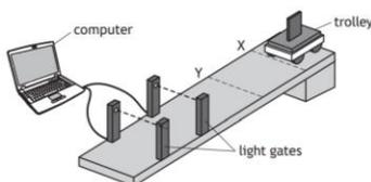
The computer displays the acceleration and average velocity of the trolley between the light gates. The trolley is now released from rest at point Y.
